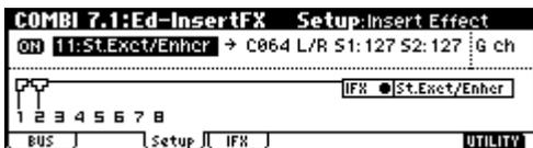
The Setup page displays the state of the routing and insert effect settings. "BUS Select" settings can also be made in this page. Use the cursor keys [▲], [←], [▼], [→] to select the timbre, and use the [INC]/[DEC] keys to make the setting.
