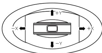
**JS(+X):** Move the joystick toward the right to apply an effect. Normally this is used to control the pitch (bend up).
