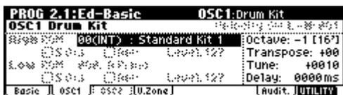
In the Basic (Prog Basic) page, set “**Mode (Oscillator Mode)**” to **Drums**. When this is set to **Drums**, you will be able to create a drum program. This will select a **drum kit** instead of a multisample. This instrument provides sixteen factory preset drum kits that are suitable for a wide variety of music. (≡Drumkit name, VNL)
