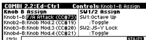
For each combination, you can specify the functions of the B-mode functions of REALTIME CONTROLS knobs [1]–[4], and the [SW1] and [SW2.] (see p.115, PG p.36, 220, 221)
