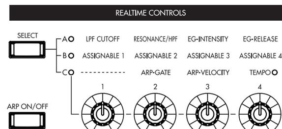
Use the [SELECT] key to select realtime controller mode A/B/C, and use knobs [1]-[4] to control the tone, effects, MIDI control changes, and arpeggiator etc. while you perform. (p.24, 26)
