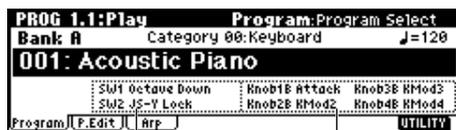
Functions assigned to the [SW1] and [SW2] keys      Functions assigned to Knob1–4
