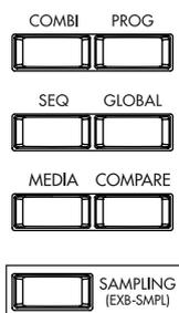
These keys are used to enter each mode. Pressing a key will enter the corresponding mode (the key will light). (p.14)
