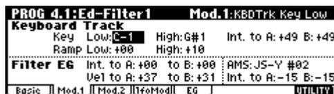
Controllers and the filter EG can be used to modulate the filter cutoff frequency that was specified in the Basic page. By using a controller to vary the tone or by using an EG to create time-varying changes, you can add a rich variety of tonal change to the sound.
