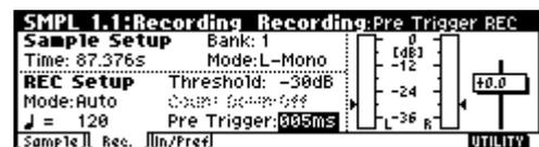
③ In REC Setup, set "Mode (REC Mode)" to "Auto," and set "Threshold" to -30.
