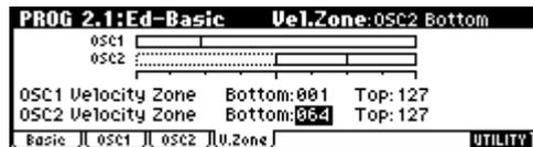
Here you can specify the range of velocities that will sound oscillators 1 and 2. In the example shown above, the velocity ranges are as follows.
