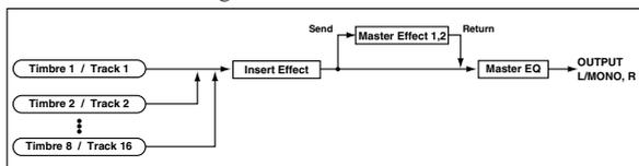
In **Sampling mode** (if the separately sold EXB-SMPL option is installed), the sound of an external source that is input from AUDIO INPUT 1 and 2 can be processed by the **insert effect** as the sound is sampled. Sampling mode settings are made by the "Input 1" and "Input 2" parameters of the SMPL 1.1: Recording, Input/Pref page. The settings here are valid only within Sampling mode.
