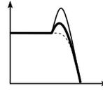
Adjusting the cutoff frequency of the high-pass filter will modify the thickness of the sound from which the low frequency range has been filtered out.
