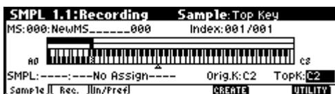
**note** If you want to create a new multisample, use the numeric keys to input the number of the multisample that you want to create, and press the [ENTER] key.
