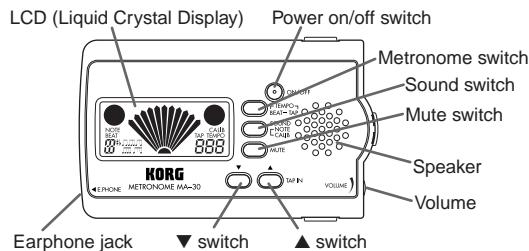
Press the power on/off switch to turn on the power.
