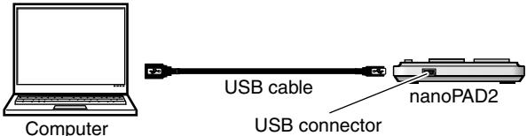
1. Use a USB cable to connect the nanoPAD2 to a USB port on your computer. The power to the nanoPAD2 will turn on and the power LED will light up.
