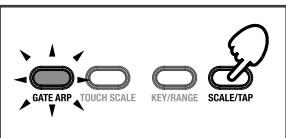
You can set the tempo of the Gate Arpeggiator by pressing the SCALE/TAP button several times at the tempo that you desire. The GATE ARP button indicator will flash in sync with the tempo. Pressing the SCALE/TAP button twice or more will change the tempo accordingly. The more times you press the button, the more precisely you can set the tempo.
