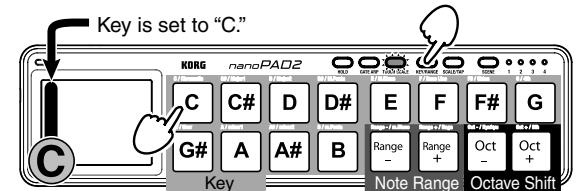
While pressing and holding down the KEY/RANGE button, press the trigger pad where the desired Key, Note Range, or Octave Shift setting is assigned.
