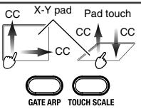
X and Y-axis: Moving your fingers along the X or Y-axis transmits control change messages.
