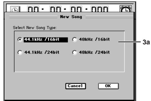
3a. Song Type [44.1kHz/16bit, 48kHz/16bit, 44.1kHz/24bit, 48kHz/24bit]
