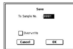
In “**To Sample No.**,” specify the save destination sample number. By default, an unused sample number will be selected. If “**Overwrite**” is checked, this cannot be selected.
