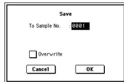
In “**To Sample No.**,” specify the save destination sample number. By default, an unused sample number will be selected. If “**Overwrite**” is checked, this cannot be set. If you wish to delete the original sample data and overwrite it with the edited sample, check “**Overwrite**.”
