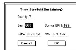
⑤ Set “Quality” to specify the desired audio quality of the sample produce by Time Stretch. The range is 0–7. Although it will depend on the sample, higher settings will produce better results. However, be aware that higher settings will also require a longer time to execute. Since you can try this as many times as you like, you should normally start with about 4, and raise or lower the setting gradually.
