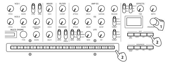
**2.** Hold down one of the buttons from 1–16 while keeping the SHIFT button pressed. The program will be registered as a favorite program, and "Registered to Favorite" will be shown in the display.
