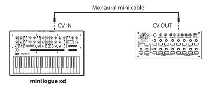
Configure the CV IN jack settings on the minilogue xd from "Button 5 (CV INPUT)" (p.33). See the owner's manuals of each respective external device to synchronize.
