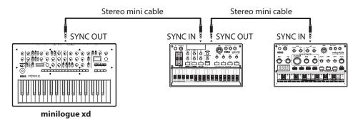
Use the same settings for "Sync Out Unit" (p.41) on this minilogue xd and "Sync In Unit" on the first external device to sync. Similarly, use the same settings for "Sync In Unit" on the second external device to sync.
