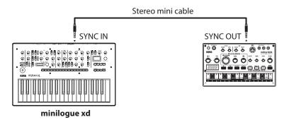
Use the same settings for "Sync In Unit" (p.41) on this minilogue xd and "Sync Out Unit" on the external device. Similarly, use the same settings for both the "Sync In Polarity" (p.41) and the "Sync Out Polarity" on the external device.
