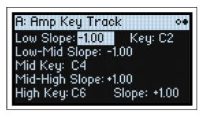
Keyboard tracking ("Key Track") changes the volume as you play up and down the keyboard. This may be used to make the volume more consistent, or to create special effects.
