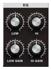
This is a two-band equalizer. Use EQ FREQ to specify the frequency that you want to adjust, and use EQ GAIN to adjust the gain of each frequency band.
