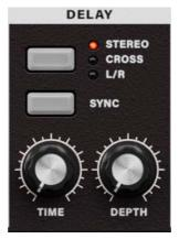
The delay effect simulates the delays that occur when sound travels through air. "TYPE" selects the type of delay effect. "DELAY DEPTH" sets the delay depth and the amount of feedback. "TEMPO SYNC" specifies whether the delay time will be synchronized to the tempo set by the arpeggiator or by an external MIDI clock.
