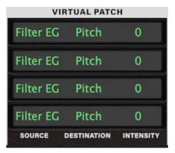
The microKORG provides four Virtual Patch routes that let you create more sophisticated sounds. Each patch lets you select a modulation source "SOURCE" and modulation destination "DESTINATION", and specify the intensity of modulation "MOD INT". By using various patchings you can create a wide variety of changes in the sound.
