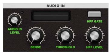
These parameters adjust the input from AUDIO IN (the modulator).
