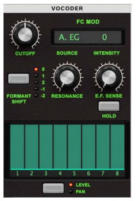
By using "FORMANT SHIFT" and "CUTOFF" to shift the cutoff frequency of each band pass filter of the carrier (the "synthesis filter"), you can raise or lower the frequency response while maintaining the character of the modulator, thus varying the character of the vocoder output. Both of these knobs do the same thing, and have the same range.
