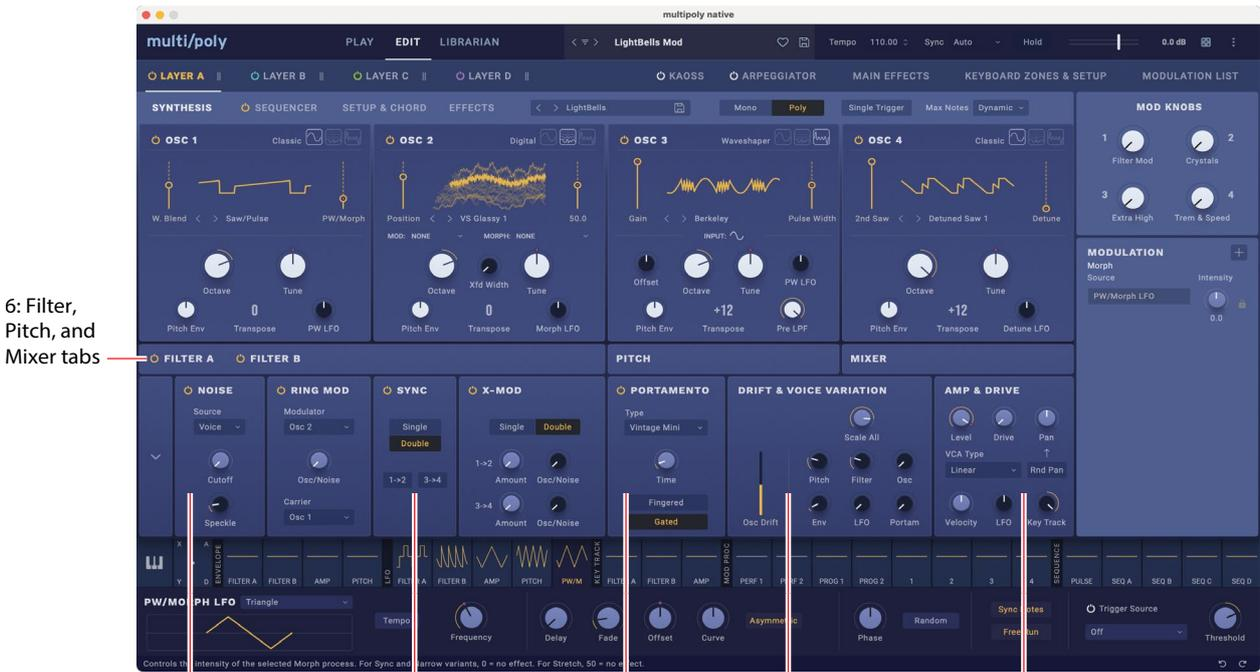
1: Noise Generator 2: Ring Mod, Sync & X-Mod 3: Portamento 4: Drift & Voice Variation 5: Amp & Drive
