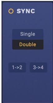
When **Sync** is *On*, the sync leader (e.g. Oscillator 1) controls the pitch of the sync follower(s) (e.g. Oscillator 2). Every time that the sync leader begins a new cycle—the instant that it passes through zero going from negative to positive—the sync follower snaps back to the start of its waveform. Changing or modulating the follower's frequency changes its timbre, instead of its pitch.
