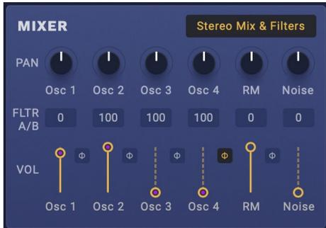
The Mixer has six inputs: Oscillators 1, 2, 3, and 4, the Ring Modulator, and the Noise Generator. Each input includes Level, Pan, and Filter A/B Balance, and all but the Noise Generator also include a Polarity switch.
