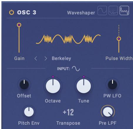
This is a west-coast style waveshaper/“wavefolder” oscillator, with some special twists. A sine or triangle wave goes into a Waveshaper, with a wide selection of tables.
