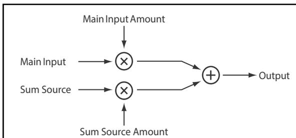
Sum adds two modulation sources together. This is useful if you want to process the combination of two or more signals: for instance, to merge an LFO and an envelope, and then smooth the result.
