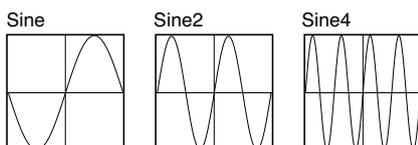
With sine wave input, these tables produce output similar to a simple FM pair with the Carrier:Modulator ratio set to 0:1. **Gain** functions like the FM input level, and responds well to modulation.
