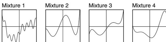
*Mixture 1, 2, 3, and 4:* With sine wave input, these four tables create a bunch of different harmonics at different amplitudes, like FM or organ stops.
