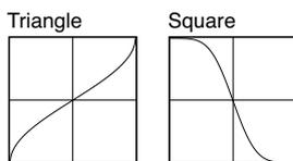
**Triangle:** With sine input and maximum **Gain**, this table creates a triangle waveform. If you just want to create a triangle waveform, the *Classic* and *Digital* oscillators may sound a little better, but this table allows you to use **Gain** and **Offset** in creative ways. For more mellow, sine-like tones, reduce the **Gain**; for sharper timbres, increase it.
