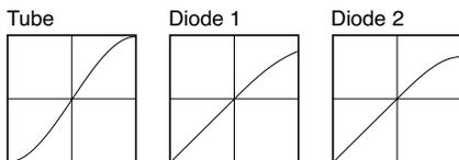
*Tube:* This is a soft-clipping table, for simulating analog saturation. **Gain** controls the amount of clipping; **Offset** controls symmetry, like DC offset into a VCA.
