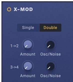
When X-Mod is On, the X-Mod leader (e.g. Oscillator 1) modulates the frequency of the X-Mod follower(s) (e.g. Oscillator 2). This results in a series of complex non-harmonic “sum and difference” frequencies above and below the root pitch, called side-bands. These side-bands can create metallic sounds, like bells or gongs.
