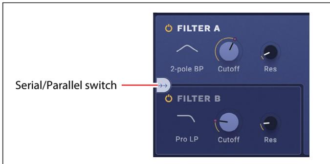
There are two filters, Filter A and Filter B. They can be arranged either in parallel, with separate paths through each filter, or in series, with Filter A feeding into Filter B. **Filter A/ B Balance**, described below, controls signal routing to the filters.
