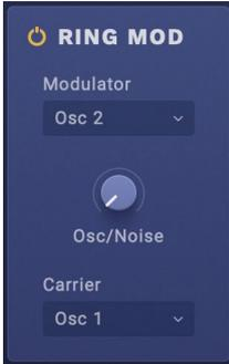
Ring Modulation modulates the volume of one signal (the Carrier) with another (the Modulator). When the frequencies of the Carrier and the Modulator are the same, the Ring Modulator produces steady, constant waveforms. When the two are detuned, it produces more movement and overtones.
