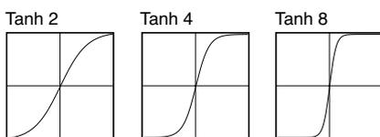
*Tanh2, 4, and 8:* These create soft clipping, similar to the Step. Vary the **Gain** to control the amount of distortion. 2, 4, and 8 produce increasing amounts of clipping. Maximum **Gain** will produce output similar to a soft-edged square wave.
