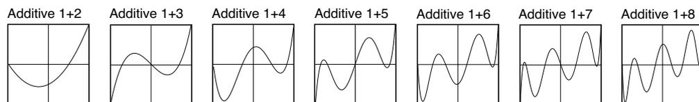
The “*Additive 1+*” group all produce the fundamental and an additional harmonic at equal amplitude.
