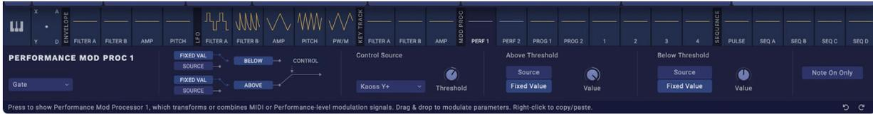
Modulation Processors transform a modulation signal to make it into something new. The original modulation signal also remains available. There are six Modulation Processors per Program, plus two for the Performance as a whole.
