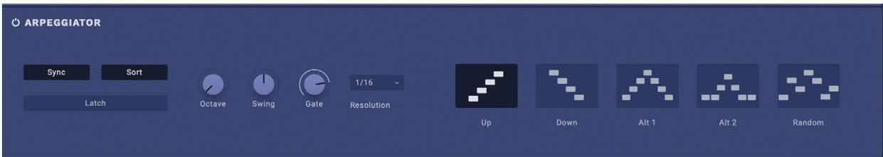
The Arpeggiator controls all four Layers; see “Structure” on page 1. It’s particularly effective in conjunction with Layer Rotate, so that each generated note plays a different Layer, or with Note Advance, so that each generated note starts on a new step in the Lane.
