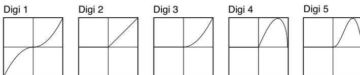
*Digi 1 through 5:* With maximum **Gain**, these produce waveforms similar to those of classic 4-operator FM synths (original TX waveforms 2, 3, 4, 7, and 8, respectively). Reduce **Gain** for a more sine-like sound.
