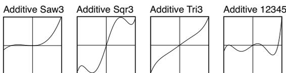
While the Additive tables can produce interesting results with any input signal, they produce the described results only with Sine input and maximum **Gain**. Reducing the **Gain** will diminish the level of the additive harmonics, making the result sound more like the original sine. Dynamic modulation of **Gain** may sound similar to a filter opening and closing.
