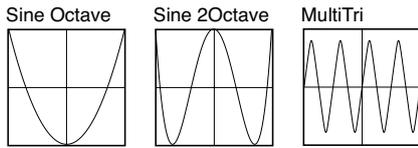
*Sine Octave:* With maximum **Gain**, this produces a sine wave one octave higher than the input, and clips above 0 dB.
