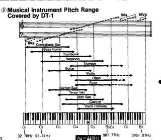
●In the SLOW or FAST mode, the DT-1 can measure the pitch of inputs over a 7-octave range from C1 to B7, as shown in the chart. In the SOUND mode, the DT-1 can generate reference tones over a range of four octaves from C2 to B5.
