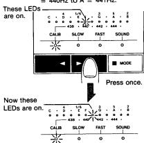
Note: Standard pitch returns to 440Hz when power is turned on, regardless of the setting in effect when the power was turned off.
