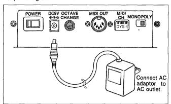
Connecting MIDI OUT jack: All data from the MPK-130 is sent through the MIDI OUT jack. Using the supplied MIDI cable, connect the MPK-130's MIDI OUT to the MIDI IN jack of the synthesizer or expander module to be used.
