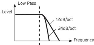
This is a filter that cuts the high-frequency region above the cutoff frequency. This is the most common type of filter, and is used to cut part of the overtone components, making an originally bright timbre sound more mellow (darker). When the "Filter Type" is Low Pass Resonance, the cutoff will have a steeper slope.
