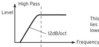
This filter cuts the low-frequency range that lies below the cutoff frequency. By cutting the lower overtones, it lightens the tone.
