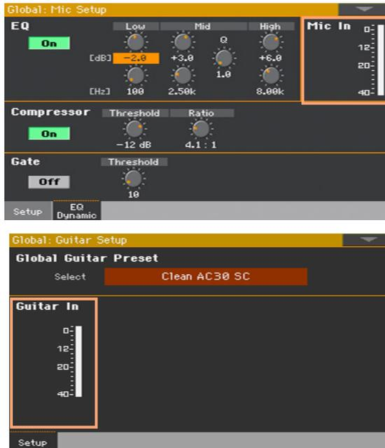
With a microphone or line audio device, keep the level so that this indicator remains green most of the time, with orange appearing at signal peaks. Never go to red.
