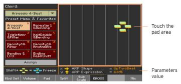
Depending on the selected preset, the grid in the KAOSS pad will change. Each cell corresponds to a block of values (also called a step). The lighter grey cells are the default value for the corresponding parameter.
