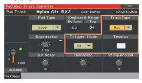
2 Press the corresponding button on the control panel to select one of the Style Elements (VARIATION1 ... ENDING3). Use the Track Type parameter to set the type of the corresponding track.
