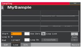
The loop is a cycling portion of a sampled sound. Looping is a technique used to reduce the sampling time, cycling a portion of the sound to create the sustaining phase of the sound. After the attack stage, most sounds repeat the same waveform during their sustain stage.
