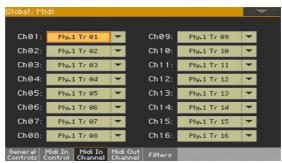
Use the Channel pop-up menus to assign an instrument's track to each MIDI channel.
