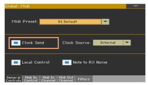
Select the Clock Send parameter to send the internal MIDI Clock to the MIDI IN and USB ports.
