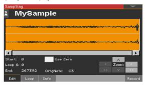
This page allows you to cut, trim or normalize a sample, as well as edit the loop points. The sample can be played over the full keyboard.
