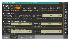
When the filter type is Low Pass Resonance, the parameters for filter B will not be editable (dimmed).
