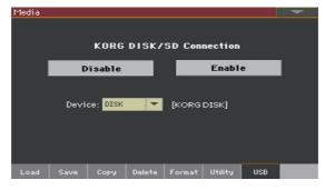
While USB file transfer is enabled, you cannot access other functions on Pa1000. MIDI Over USB is also disabled.
