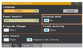
Select the Display Hold checkbox to let the Select windows remain open until you press the EXIT button. Deselect it to let the Select windows automatically close after you choose an element.
