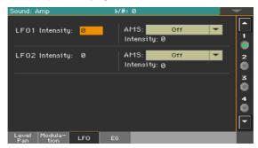
Use the LFO 1/2 > Intensity parameters (-99...+99) to adjusts the effect of the cyclic modulation that LFO 1/2 (set in the LFO > LFO 1 and LFO 2 pages) will apply on the amp EG. Negative (-) settings will invert the phase.
