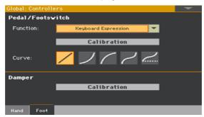
Touch the Calibration button in the area of the pedal to calibrate, to make the Damper & Pedal/Footswitch Calibration dialog appear.
