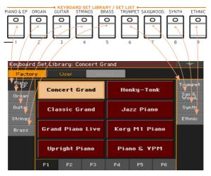
To choose one of the available pages in the selected Keyboard Set group, either touch one of the P1...P6 tabs at the bottom of the window, or repeatedly press the button of the selected group of Keyboard Sets in the KEYBOARD SET LIBRARY section of the control panel.
