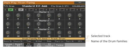
On each Drum Family strip, use the Master knobs to control the level of the direct (dry) signal sent to the corresponding FX processor (inside the selected FX group).
