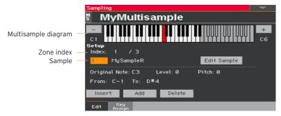
In this page you will assign the sample(s) to a multisample. Assign each sample to a different keyboard zone.
