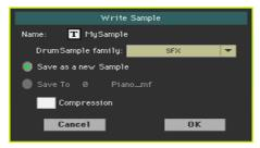
2 While in this dialog, select the Compression checkbox, to reduce the size of the sample up to a half of its original size. Please note that compression may require a long time.
