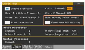
2 Use the Note Velocity Value parameter to set a fixed Note On velocity value for all the notes received via MIDI. This is useful when playing Pa1000 with an organ or a MIDI accordion, often sending a fixed velocity value.
