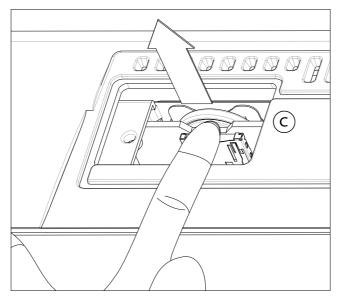
4 Insert the new battery (d) into the empty battery slot, being sure the positive (+) side is facing up. Be very careful not to let it fall inside the instrument.
