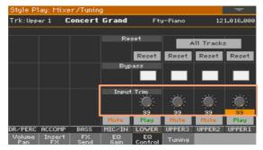
2 Use the Input Trim knobs to attenuate the level of the signal passing through the equalizer.
