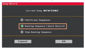
3 Choose the Backing Sequence (Quick Record) option and touch OK to access the Backing Sequence Record page.
