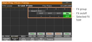
While in the Insert FX page, touch the name of the selected effect type, or the 'x' symbol under the On/Off button, to open the FX Edit page.
