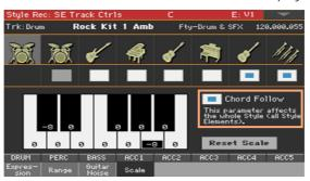
Use the Chord Follow checkbox to turn the option on or off. See the table above to see how it works.
