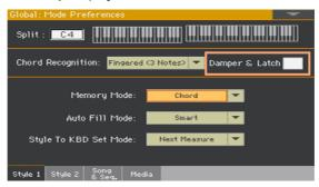
Select the Damper&Latch checkbox, to make the recognized chord be held 2 for as long as the Damper pedal is kept pressed.
