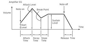
Use the Level parameters (-99...+99) to specify the volume level that will be reached at the end of the segment.
