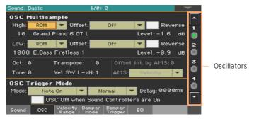
If you cannot see the desired oscillator, touch the scroll arrow, until the hidden oscillator is shown in the display.
