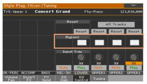
2 Select the Bypass checkbox on the mixer channel you want to exclude from equalization. Deselect it to activate the EQ again.
