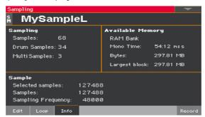
Use the Sampling area to get information on the number of samples, drum samples and multisamples in the Sampling memory.
