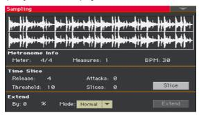
Adjust the Extend > By parameter to set the length of the 'tail' added to the samples (in percentage). A setting of 20-30% is usually suitable to most grooves.
