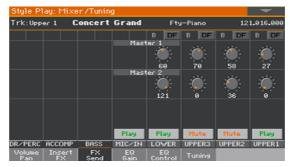
On each mixer channel, use the Master knobs to control the level of the direct (dry) signal sent to the corresponding FX processor (inside the selected FX group).
