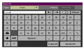
When finished entering the name, touch the Search button. After a while, the 2 list of items found will start showing on the display.
