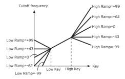
Set the Intensity to A and Intensity to B parameters (-99...+99) to specify the depth and direction of the changes applied to filters A and B.
