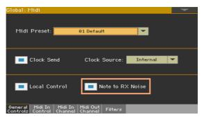
When this parameter is turned on, notes received from the MIDI IN or USB ports, or performed by the internal Player, in the RX Noises range, are recognized and converted to RX Noises.
