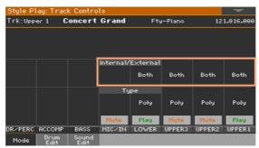
Use the Internal/External parameter to connect the corresponding part/ track to the internal and/or external sound generation.
