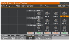
Keep the Gain knob held on the screen, and move it to the desired level. As an alternative, use the VALUE control to change the value of the selected knob.
