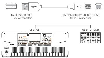
You can use an USB hub to connect more devices to the same USB HOST port (for example, an external keyboard and a breath controller).
