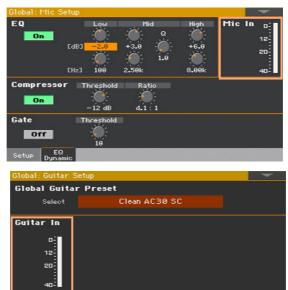
With a microphone or line audio device, keep the level so that this indicator remains green most of the time, with orange appearing at signal peaks. Never go to red.
