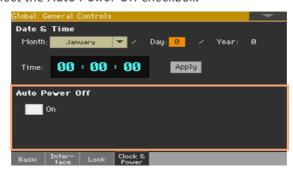
When this parameter is checked, a few minutes before automatic standby a message will warn you that the instrument is going to be put in standby. All unsaved data currently in editing or recording will be lost.
