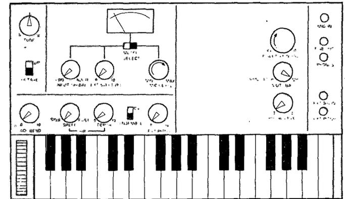
Plug a microphone into the MIC INPUT (or "BTS") jack, and connect the supplied audio cable from the FINAL OUT jack to the amp input. Turn the POWER/FINAL VOLUME knob clockwise: the meter lamp should light.
