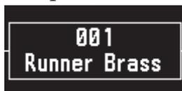
**TIP** In addition to showing Program name and number, the display can also be used as an **oscilloscope**, to show the electrical signals created by the waveform of the sound.
