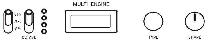
This engine operates as either a noise generator, a VPM oscillator or a user oscillator, to make a wide range of sounds not possible with analog oscillators. You can upload your own oscillator programs to the user oscillator to make sounds.
