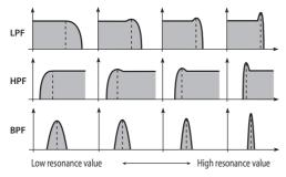
Depending on the cutoff frequency or the input audio, increasing this value may cause distortion.
