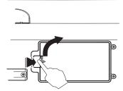
KROSS 88-key: While pressing the ||| area of the cover(a.), slide it diagonally upward (b.), and open the battery compartment (c.).
