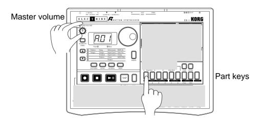
4. When you have finished making connections, turn on the power. Slightly raise the master volume of the ER-1, and strike the part keys (PERCUSSION SYNTHESIZER 1...4) to check whether connections have been made correctly. Use the master volume of the ER-1 and the gain and fader controls of your mixer or powered monitor system to adjust the volume to an appropriate level.
