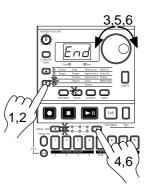
If you wish to view the order of patterns in the song, or to reselect the pattern for a specific position, make the parameter select LEDs indicate Pattern. Each time you press a select key, you will move to the next or previous position. You can use the dial to change the pattern number that is displayed.
