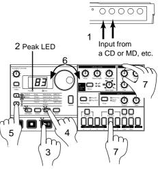
The input sound will be heard while you press the Audio In part key. The Audio In parts that are recorded in a pattern or song do not produce the sound that was being input when the parts were being recorded; they simply allow the sound that is received in the audio input at that moment to be heard from when the trigger is turned on, for the duration set by the **Decay** knob.
