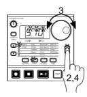
If the Global mode Memory Protect setting is on, it will not be possible to write the data. In this case, turn off the Global mode Memory Protect setting before you execute the Write operation.
