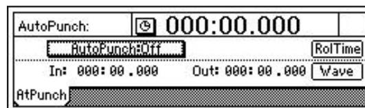
You can also set In / Out times by selecting the "Wave" button in the Auto Punch page - a great feature that lets you set precise punch in / out times while viewing a waveform display. And you can easily set Pre and Post-roll times to specify playback time before and after recording.
