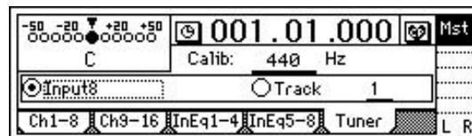
1. **[STOP]** playback, then press **[INPUT]** until you select the "Tuner" tab. Here, you can tune an instrument connected to the **GUITAR IN** or **INPUT1** jack.
