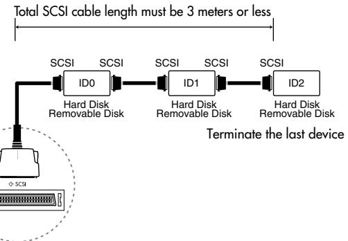
⑤ Turn on the power of the external SCSI device(s), and then turn on the power of the instrument (in which the EXB-SMPL is installed).
