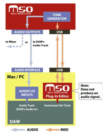
*Note*: Because the M50 Plug-In Editor does not handle audio signals, you can't insert a plug-in effect into the channel of the track in which the M50 Plug-In Editor is inserted, or send its audio signal via a send or bus.
