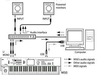
*Note:* For details on creating audio tracks, MIDI tracks, and plug-in instrument tracks, and on how to perform operations and make settings in your host application, refer to the host application's owner's manual.
