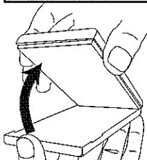
While pressing the area marked OPEN on both sides, open the case, and insert the batteries being careful to observe the correct polarity. Battery life may differ according to the conditions of use. If the unit malfunctions, and turning the power OFF and then ON does not resolve the problem, remove and then reinstall the batteries.
