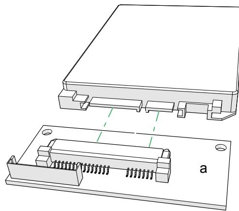
**3** Use two screws (c) to secure the hard disk drive (not supplied with the kit) to the interface board (a) and to the metal support (b), as shown in the illustration. Use the two screws (d) to secure the hard disk to the support (b).
