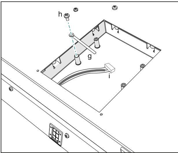
**6** Connect the data cable (i) to the dedicated connector on the interface board (a).
