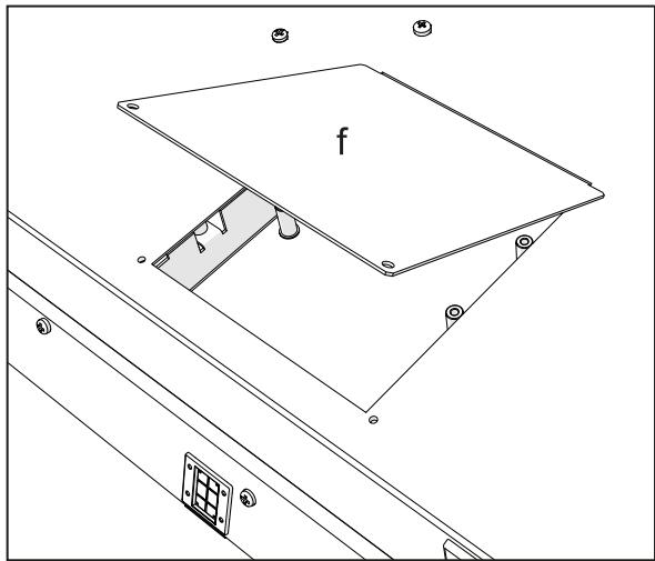
**5** Disconnect the data cable (i) from the fixing clip (g), and remove the clip (g) by unscrewing the fixing screw (h).
