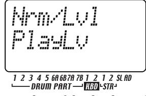
4. The upper line of the display indicates "Play Lvl," and the lower line indicates "0 dB" or "+12 dB." Use the dial to select the desired setting, and press step key 11 once again to set the Play Level (key 11 will go dark).
