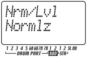
3. The upper line of the display indicates "Nrm/Lvl," and the lower line indicates "Normlz" or "PlayLv." Use the dial to select "Normlz," and press step key 11 once again.
