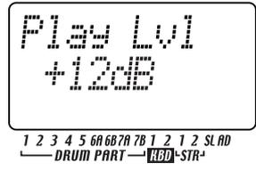
**note** Samples that are set to "+12 dB" are indicated by a "+" symbol added to their displayed sample number.
