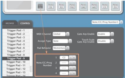
To send chords, assign the chord notes to each pad. Assign a different chord of a chord sequence to each pad.
