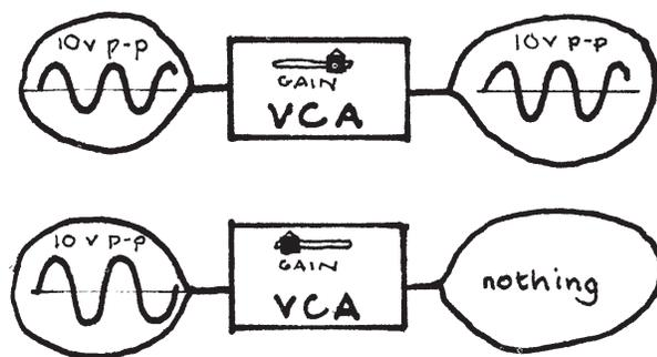
4.13 The VOLTAGE CONTROLLED AMPLIFIER has a maximum gain of unity and a dynamic range of 100Db. With the INITIAL GAIN control at maximum, and with no control input, the VCA will pass with unchanged amplitude any signal presented to its signal input. On the other hand, with the INITIAL GAIN control at minimum, no signal will pass through the amplifier at all unless some positive voltage is present at one or both of its control-voltage inputs.
