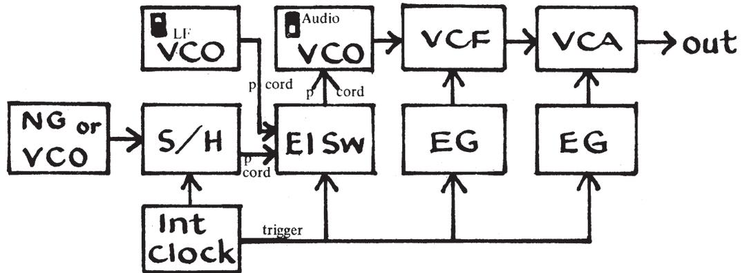
You might, if you wish, begin with a slightly simplified patch ; omit the S/H circuit and feed two VCO's directly into the Electronic Switch. Then experiment thoroughly and systematically. Go on to the patch above. Don't neglect the possibilities of audio-range switching rates; the Internal Clock is capable of rates up to about 100Hz.
