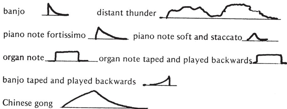
2.17 Any low-frequency waveform may be used to produce events and to give them a shape. But usually a synthesizer will have one or more devices designed specifically to generate low-frequency wave-shapes suitable for giving events a shape. These are called ENVELOPE GENERATORS or ENVELOPE TRANSIENT GENERATORS. Their output is APERIODIC (see 2.1422); instead of appearing over and over again spontaneously it appears only when the envelope generator is TRIGGERED.
