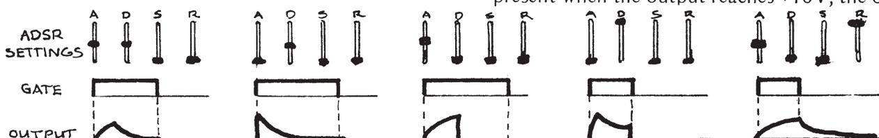
put immediately begins to decrease, at a rate determined by the setting of the INITIAL DECAY control, to a level governed by the SUSTAIN level control. The output voltage will remain at this level as long as the GATE signal remains at the generator input. When the gate signal is removed, the output voltage returns to zero at a rate determined by the FINAL RELEASE time control.
