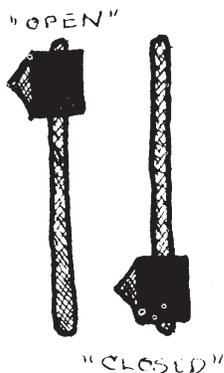
a signal through at full strength. “Closing“ the attenuator control slowly—i.e. sliding it down—gradually weakens the signal passing through it until there is no signal at all.
