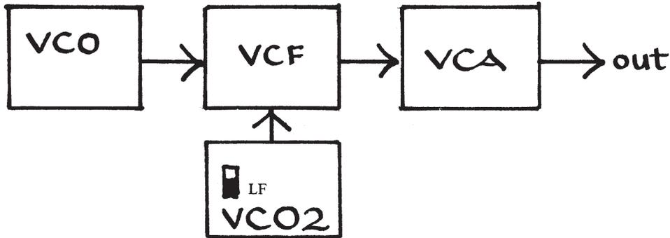
So far you've been using only pink noise as your sound source. Now close the input from the noise generator and try instead feeding an audio signal from VCO1 or VCO3 into the filter. Again take special note of the very general and basic difference between low-frequency modulation of the filter  $F_c$  and audio-frequency modulation of the filter  $F_c$ .
