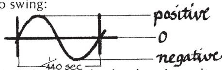
2.124 The same microphone passing its changing voltages on to an amplifier, and the amplifier feeding its output to a loudspeaker, would make the loudspeaker cone move back and forth:
