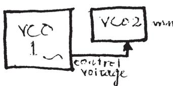
2.3 A SYNTHESIZER, then, consists of SIGNAL-GENERATING and SIGNAL-MODIFYING equipment; and some of this equipment is VOLTAGE-CONTROLLED by signals which usually are generated, and may also be modified, within the synthesizer.
