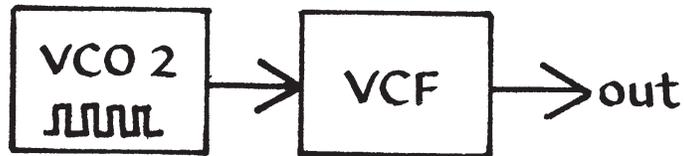
5.103 Close the VCO1-Filter input and open the VCO2-Filter input. Tune VCO2 to unison with VCO3, just for practice. Then close the VCO3-Filter input and listen to the pulse-wave output of VCO2 all by itself. This has some interesting peculiarities.
