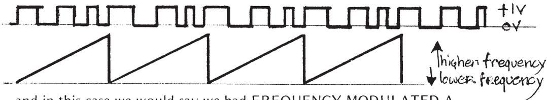
and in this case we would say we had FREQUENCY-MODULATED A 100Hz SQUARE WAVE WITH A 25Hz SAWTOOTH.
