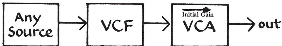
5.108 Now close the VCF-Mixer input and open the VCA-Mixer input. Open the VCF-VCA input and raise the VCA initial gain to maximum. Feed any audio signal you please into the filter; note that with the new signal path you have set up, the signal you are listening has passed from the filter through the amplifier before going into the mixer.
