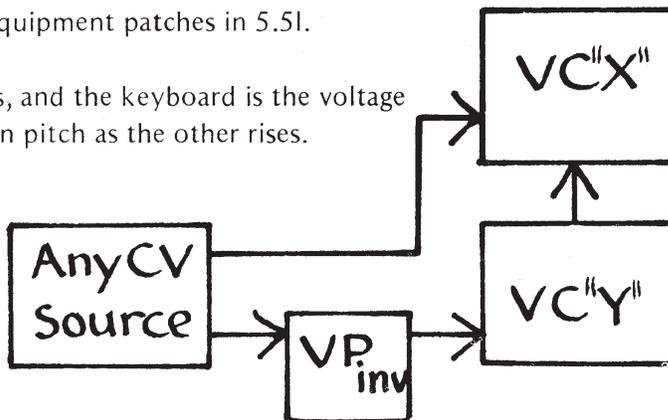
5.3 FEEDBACK LOOPS. A little-explored no-man's-land, including control of an oscillator by its own output voltage, mutual control of two oscillators each by the others output voltage, and other horrors.
