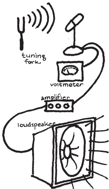
2.126 And the same generating circuit hooked up to the amplifier hooked up to the speaker would cause the same back-and-forth movement as in 2.124:
