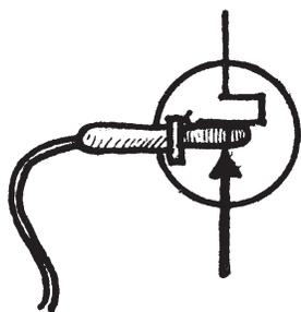
small box labelled MIC PRE-AMP. The symbol is simply a diagram of the construction of the mini-jack itself: when a plug is inserted this is what happens. THE OUTPUT FROM THE MICROPHONE PREAMP IS PREWIRED TO THE ENVELOPE FOLLOWER INPUT, AND IS AUTOMATICALLY DISCONNECTED WHENEVER A PLUG IS INSERTED INTO THE JACK INPUT TO THE ENVELOPE FOLLOWER.
