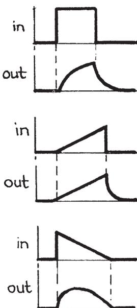
Because of its effect on audio signals the lag processor can double as a low-pass filter with maximum  $F_C$  of 1600Hz. Minimum  $F_C$  is subsonic at 1.6Hz. When it is used in this fashion, the cutoff slope is  $-6\text{Db/Octave}$  above  $F_C$ .
