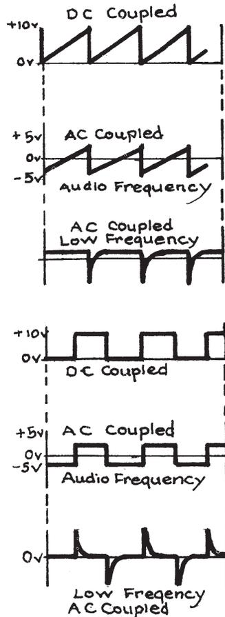
4.4 The RING MODULATOR is essentially a voltage multiplier; from two inputs A and B it produces the output function  $A \times B/5$ . The kind of transformation this effects on input signals depends to a large extent on what they are and on whether the modulator is AC or DC coupled to them. The coupling is selected by the AUDIO-DC switch at the bottom of the modulator.
