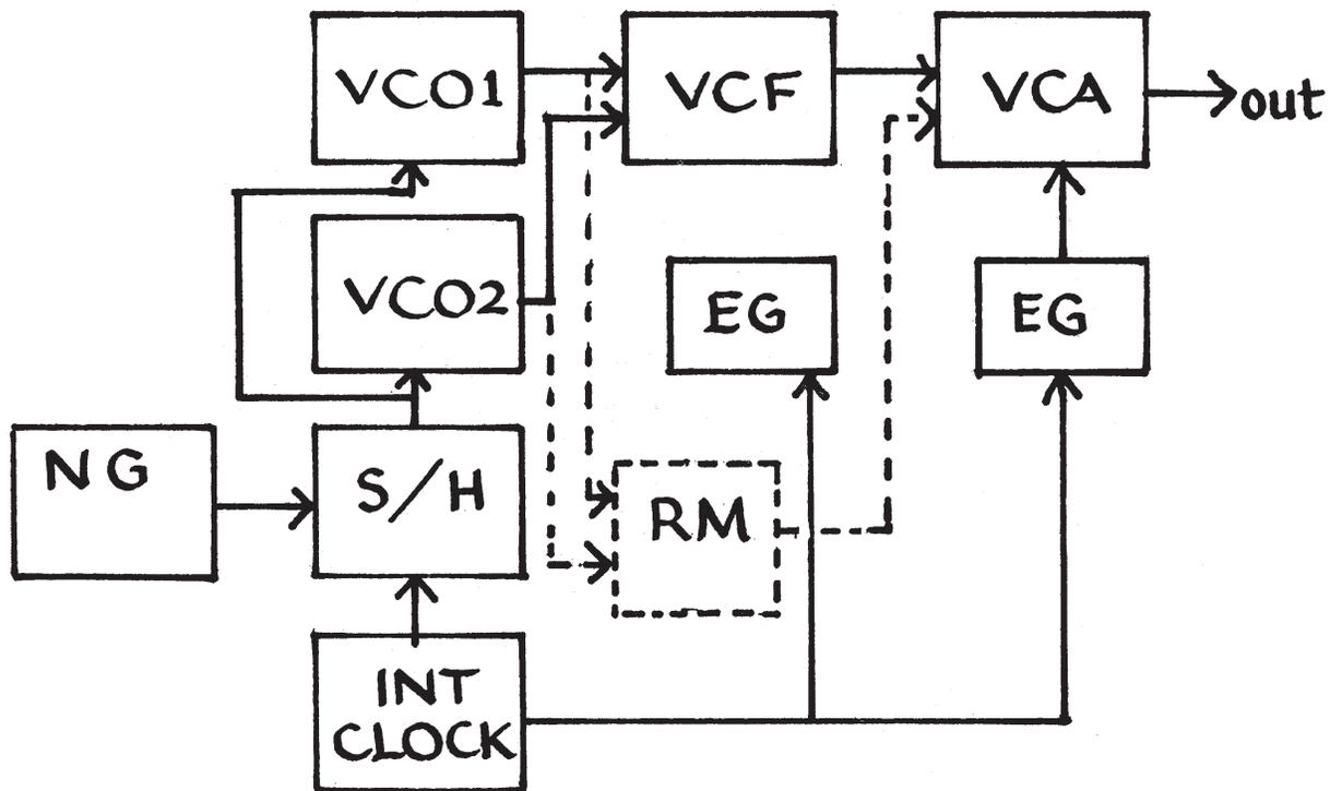
With proper control settings, the 2600 output will be a sequence of notes at random pitches, following one another at a rate determined by the Internal Clock.
