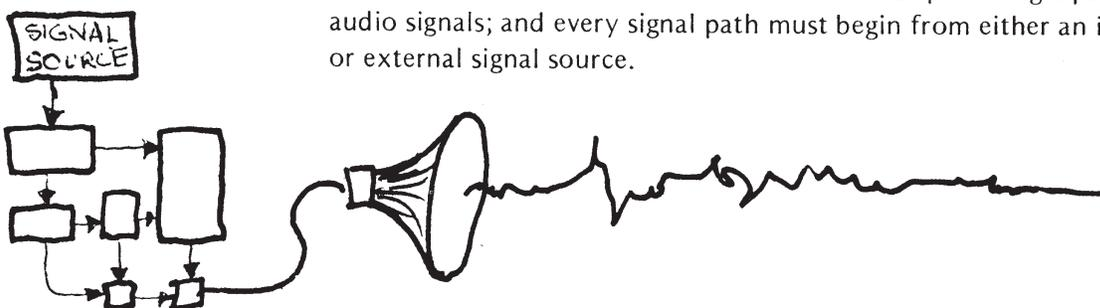
2.3311 Any signal from any device in a synthesizer may be fed directly to an external amplifier or recorder. More commonly it will be routed through other devices before reaching the synthesizer's main output channels. Several signals may be combined in a mixer, or one signal may be split to follow two different paths, which, modifying it in different ways, may later recombine.
