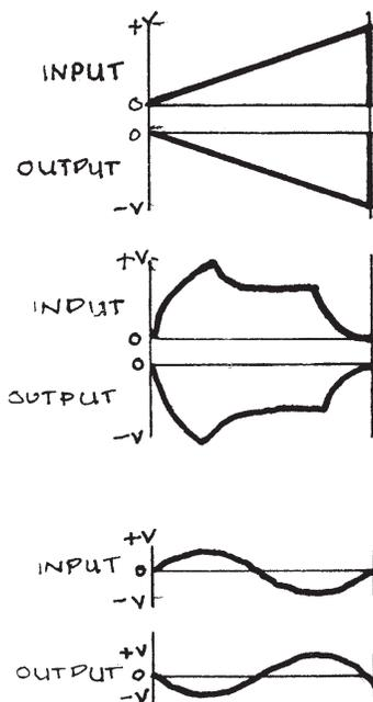
4.5 The VOLTAGE PROCESSOR section of the 2600 contains three separate processors. Two are mixing and inverting processors and the third produces a variable lag.
