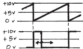
Pulse width is manually controlled by a third slider under the two frequency-control sliders and is variable from 10% to 90% duty cycle.
