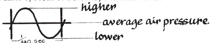
2.123 And a nearby microphone connected to a voltmeter would cause the pointer to swing:
