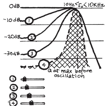
At this setting, just below the point at which oscillation begins, the filter will ring distinctly in response to any sharply defined pulse presented to its signal input. In this state it is a precise electronic analogue of any highly resonant physical
