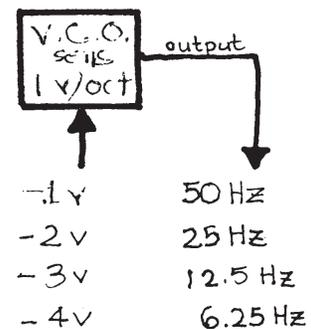
2.212 It is important to remember that VOLTAGE CONTROL is an extension of manual control; in theory anything you can do with a voltage you should be able to do with a knob, manually. IN FACT, your hands cannot move fast enough, or accurately enough, to come within miles of what a voltage signal can do with a voltage-controlled device.
