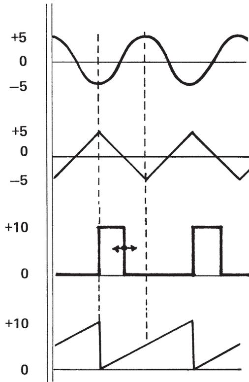
4.112 The second oscillator, VCO-2, generates SINE, SAWTOOTH, TRIANGLE, and variable width PULSE outputs at four independent outputs. Amplitude and phase relationships are given in the diagram at the left.
