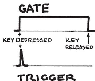
fed to the three VCO's and the VCF. In addition, the KBD CV becomes available at the output jack located in the extreme lower left corner of the 2600 main unit, and the GATE and TRIGGER outputs are available at two jacks located in the Envelope Generator section.
