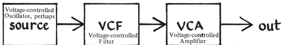
. . . in which an oscillator or noise output at some audio frequency is filtered and amplified.
