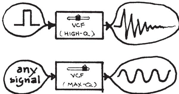
system and may be used for various percussion effects depending on its resonant frequency (identical to  $F_c$ ) and on the pulse or train of pulses exciting it.
