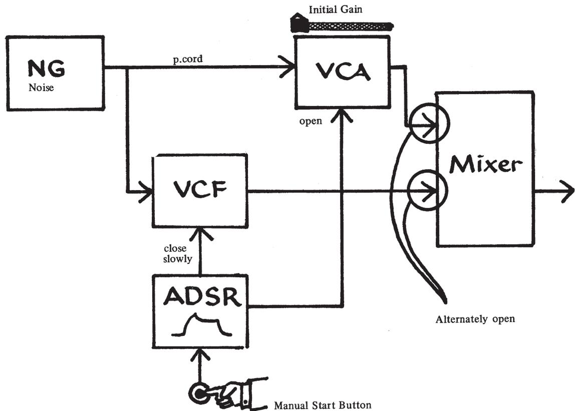
Now lower the ADSR-Filter control input attenuator to about nine-tenths of maximum and listen to the result when the ADSR generator is activated. Again at eight-tenths, and so on. As the input control voltage is attenuated, the filter is swept up to less and less of its full range and the audible output grows correspondingly duller. This is very useful technique in simulating various highly damped percussion effects such as string pizzicatos from violins, cellos, and basses.
