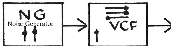
5.107 The Voltage Controlled Filter. Begin your investigation with the NG-Filter input perhaps not quite wide open—nine-tenths of maximum—the noise generator level control about two-thirds up, and the color control set for pink noise. Filter resonance at minimum and initial frequency at maximum.
