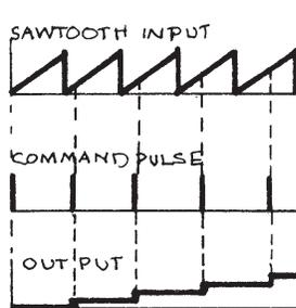
When a pulse is applied to this input, the output signal voltage immediately assumes the same value as the input signal voltage at that instant. After the sample command pulse has passed, the output signal voltage will hold its level until another sample command pulse is presented to the circuit.
