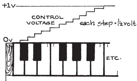
When any key is depressed, the KEYBOARD CONTROL VOLTAGE immediately assumes some value from 0V to somewhat less than +8V depending on which key is depressed and on the settings of the INTERVAL and TUNING controls at the front of the keyboard. The output will remain at this voltage until another key is depressed, even after the first key is released: a "memory" circuit in the keyboard
