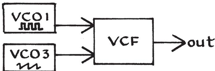
By opening both the VCO1 and VCO3 Filter inputs about halfway, you can listen to both oscillators simultaneously. Do that; if you like you can play with the resulting click patterns for a while before getting on to more serious business, namely
