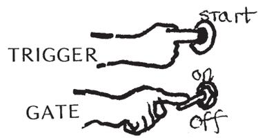
2.24 A keyboard controller for a synthesizer usually works by some combination of CONTROL VOLTAGES to signal which key is pressed down, GATES to signal the length of time a key is down, and TRIGGERS to signal the exact instant at which a key is pressed down.
