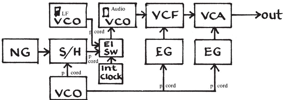
Perhaps more useful than the preceding patch. Here the gating of the Envelope Generators is independent of the Internal Clock rate for greater flexibility. Experiment primarily with the three controlling oscillators; the two low-range VCO's and the Internal Clock.
