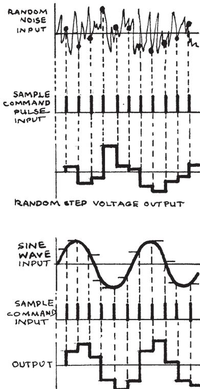
4.32 The SAMPLE AND HOLD circuit produces stepped output voltages by sampling at intervals the instantaneous value of any signal fed to its signal input. The voltages produced in this manner are useful for control of oscillator and filter frequencies and occasionally of VCA gain. Other more exotic possibilities may occur to the experienced user.
