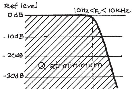
$F_C$  is controlled manually by a COARSE tuning slider (labelled INITIAL FILTER FREQUENCY) and a FINE TUNE slider.  $F_C$  may also be controlled by external voltages; the sensitivity under voltage control is 1V/Octave.
