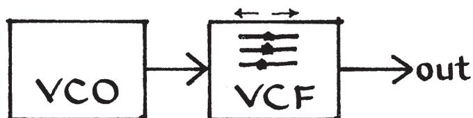
Still with all inputs closed, lower the resonance control to just below the point where the filter ceases to oscillate. At this point the filter delivers the sharpest “peaked” output it is capable of; open the NG-Filter input again and use the keyboard this time to play up and down on the filter  $F_c$ . For this experiment use pink noise.
