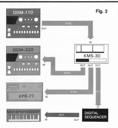
The digital sequencer will respond only to the clock and start/ stop data from the DDM-110 since that is all that is included in the MIDI signal at the KMS-30 MIDI OUT jacks.
