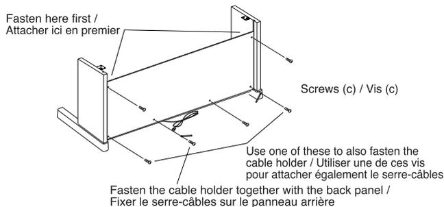
**6. Check that there are no gaps in the stand and that it is not skewed, and firmly tighten all screws, including those in step 3.**
