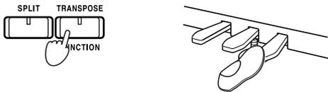
Each time you press the damper pedal, the pedal effect will be applied as shown below. At this time, the sound selector switch(s) will light to indicate which sounds will be affected by the damper pedal.
