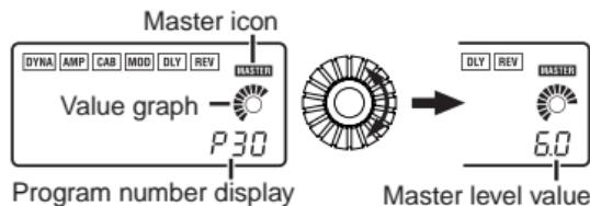
You can also adjust the settings so that the **▲/▼ buttons** will adjust the master level. (See p.16)
