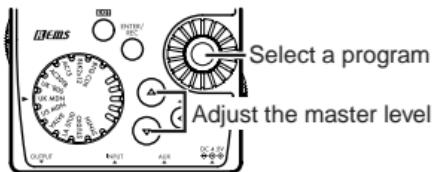
If you want to change the function of the **Value dial** so that it will adjust the master level, again, hold down the **EXIT button** once and press the **◀ button**, or turn on the power.
