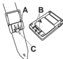
3. Press in the direction of the arrow (a) until locking tab (C) clicks into place.
