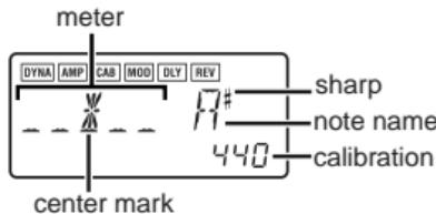
Play a single string on your guitar or bass. The LCD will show the note name and the calibration. If the pitch is more than a semitone higher than the note name, a sharp symbol will appear at the upper right of the note name.
