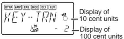
The value can be adjusted upward and downward for 3 semitones in 10 cent steps, and in semitone steps (100 cents) for the remainder of the range.
