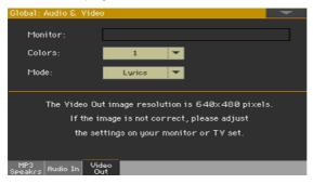
When the monitor is recognized, its name appears in the Monitor line. If it doesn't appear, check the connections.
